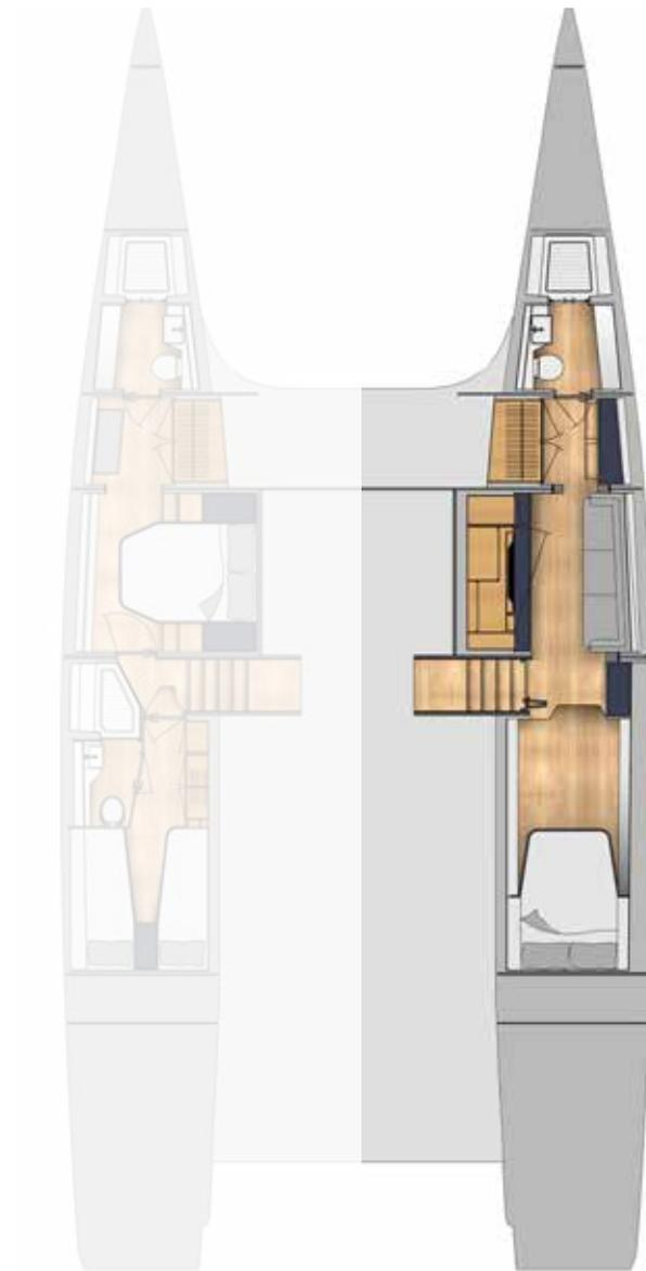
UPGRADE OPTION FOR A 4 CABIN STARBOARD HULL THAT BECOMES AN IDENTICAL REFLECTION OF THE PORT HULL.
