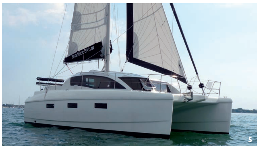
5: The shape of the coachroof and the curved chine smooth the overall lines
